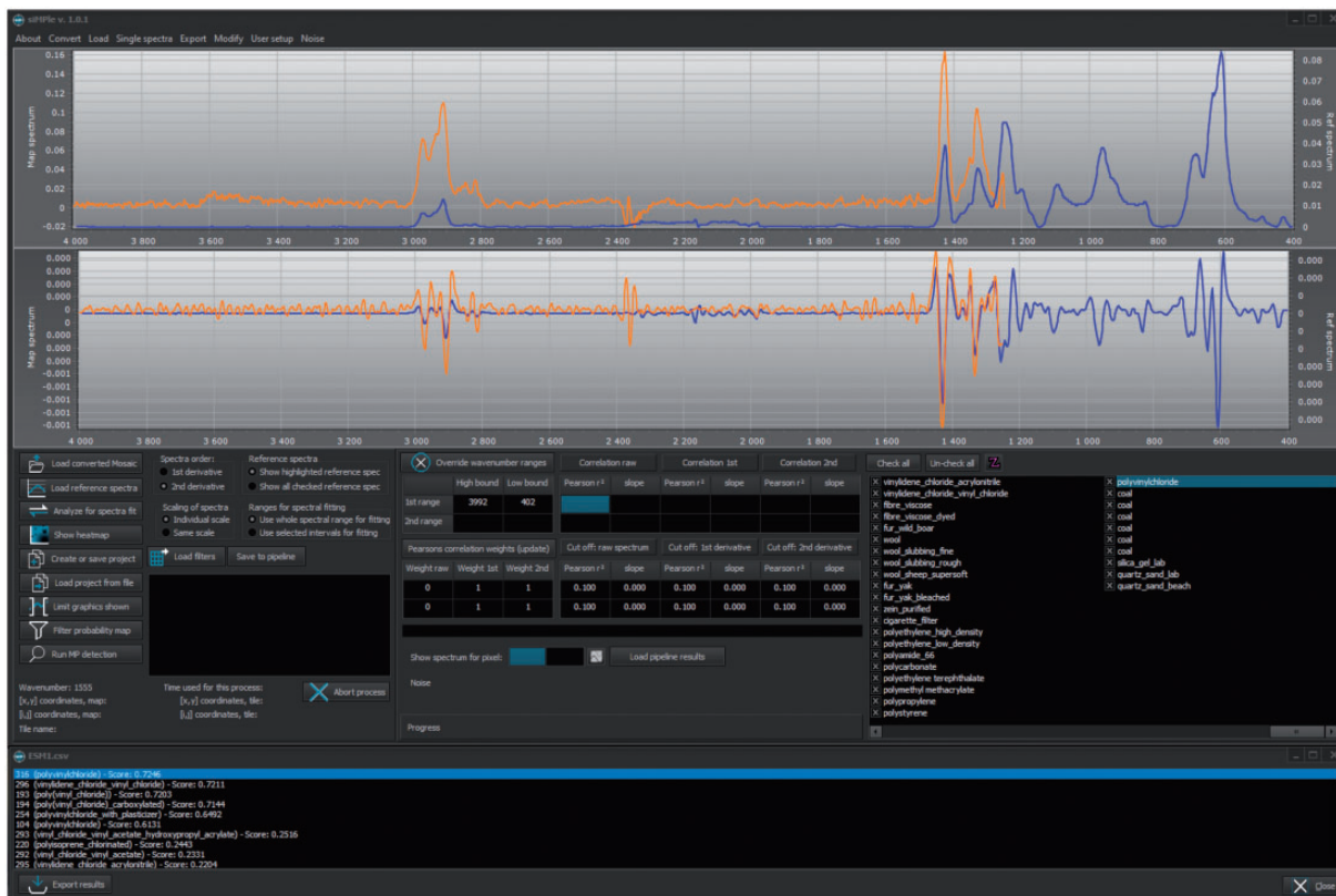
Figure 1. The software graphical user interface with a loaded reference (blue) and a sample spectrum (orange) using the Match single spectrum function of siMPle on a spectrum assigned as polyvinylchloride using ESM1.csv.
