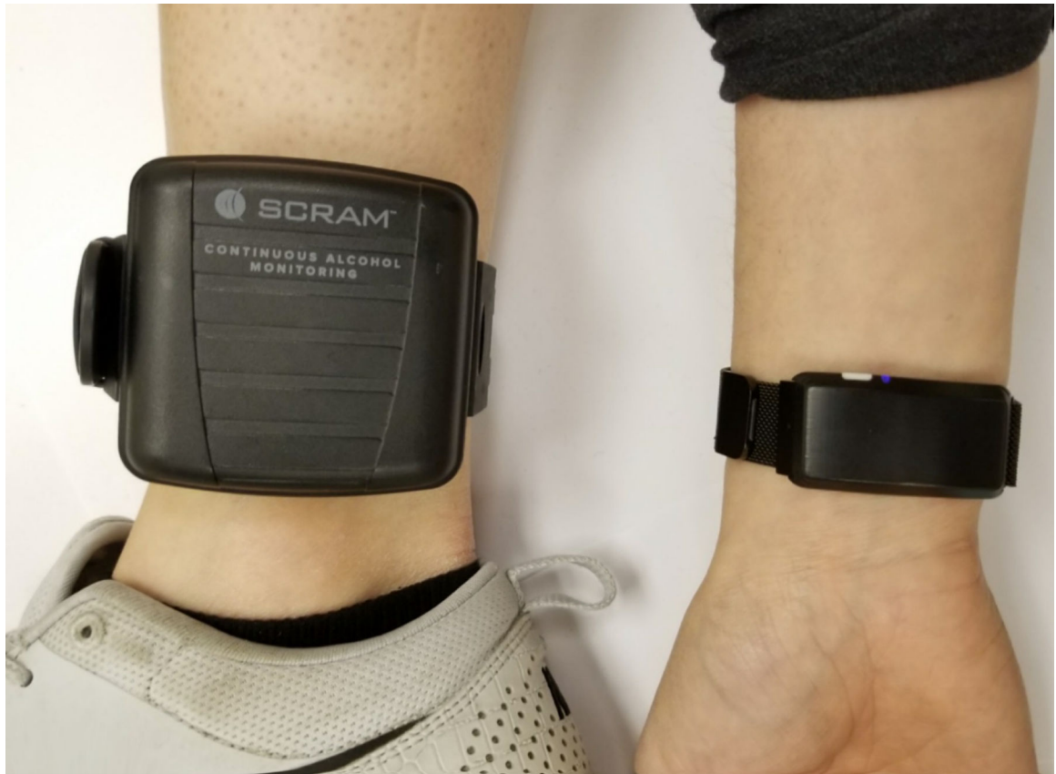
Figure 1. AMS SCRAM ankle bracelet (left) and BACtrack Skyn wrist monitor (right) displayed side-by-side. The approximate weights of the devices are 6oz (SCRAM) and 1oz (Skyn prototype).
