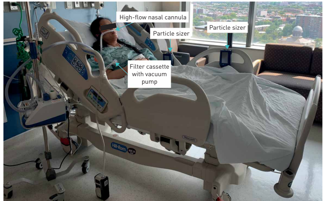
FIGURE 1 High-flow nasal cannula set-up with a filter cassette with vacuum pump for sampling room air to detect SARS-CoV-2 virus and two optical particle sizers placed longitudinally at 1 foot (30.5 cm) and 3 feet (91.5 cm) away from the patient's face to measure the aerosol concentrations.
