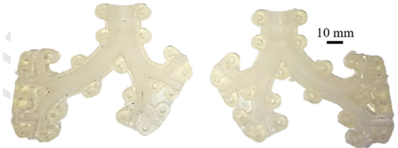
Fig. 3. Snapshot of the two halves of the 3D printed multi-generation asymmetric upper airway model, coated with Parafilm.
