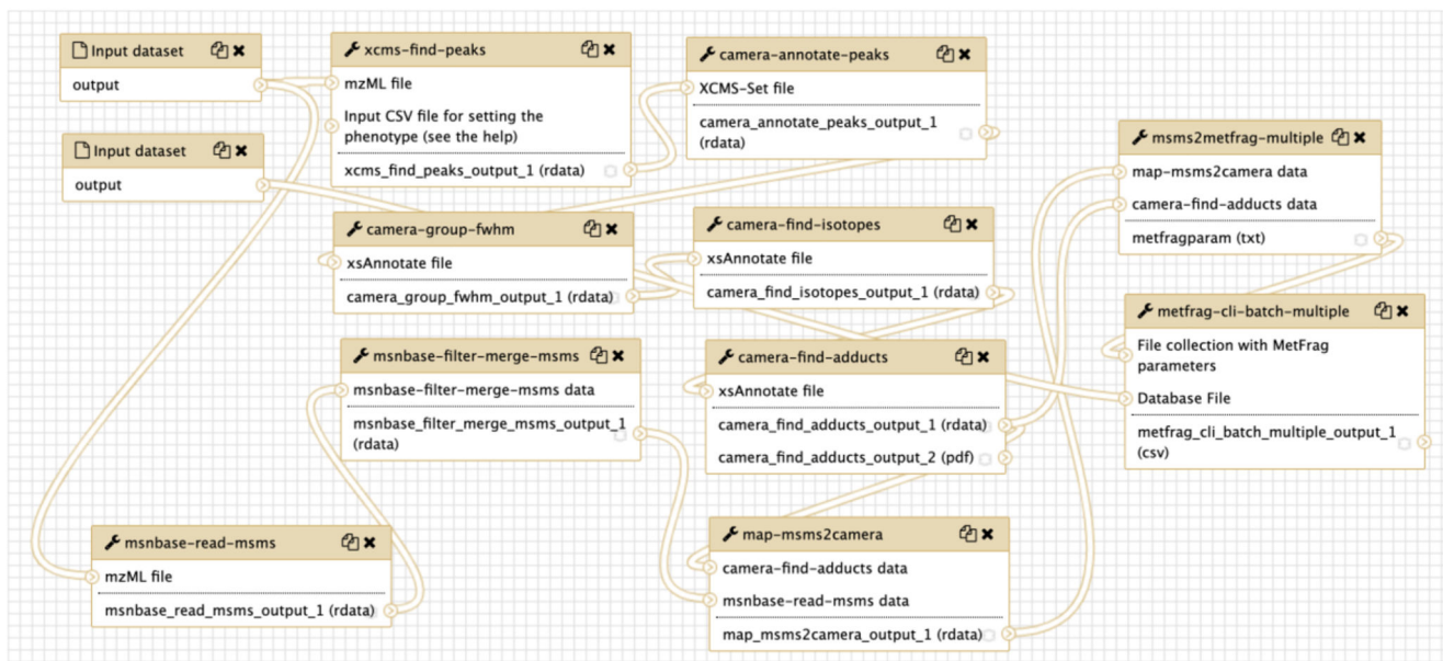
Figure 5. A Galaxy workflow from PhenoMeNal H2020, used for processing LC-MS/MS data. It integrates XCMS, CAMERA, msnbase and MetFrag for matching detected fragments to potential small molecules.
