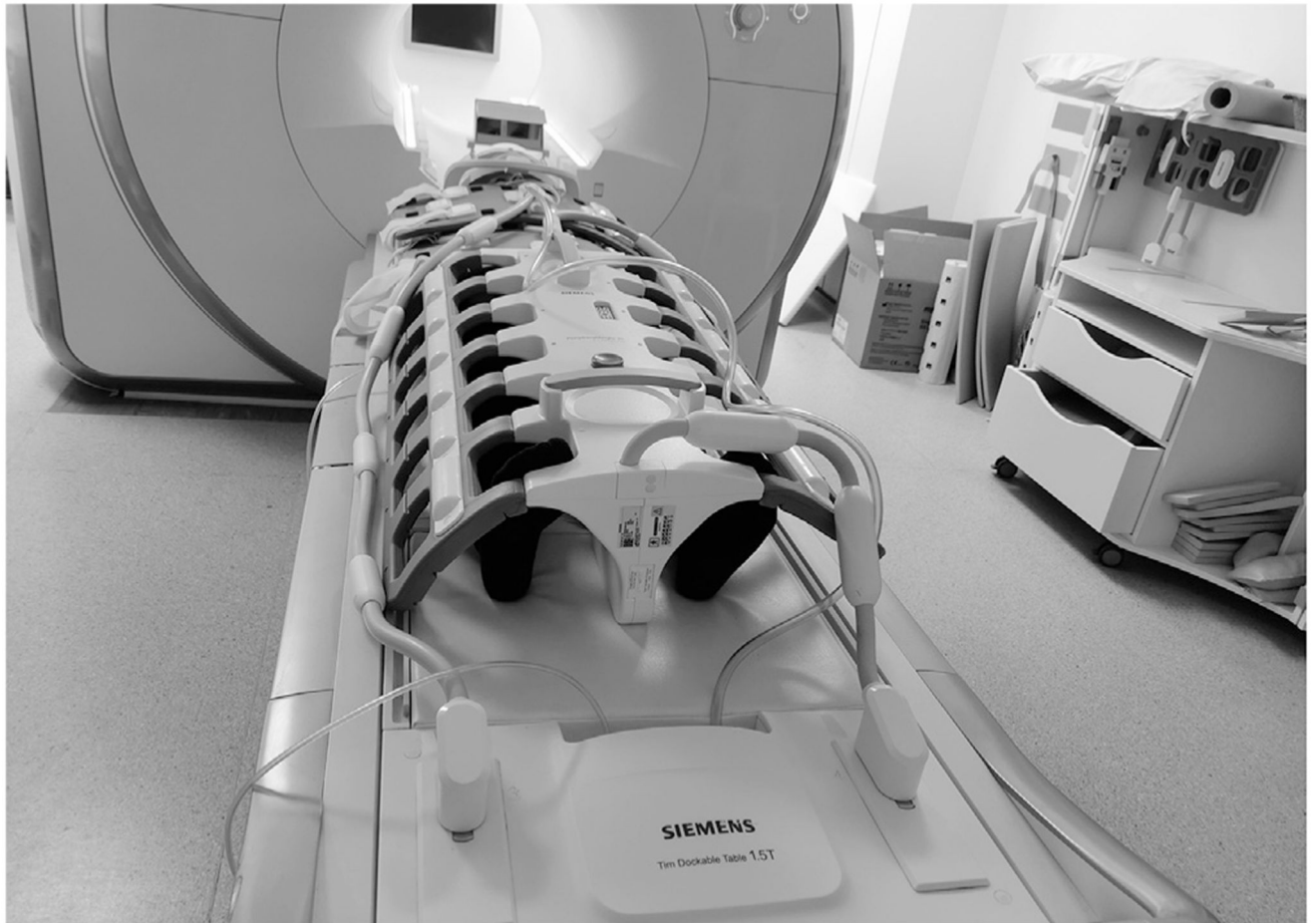
Figure 1. A volunteer wearing coils as would be worn for a whole-body magnetic resonance imaging and demonstrating the procedure.
