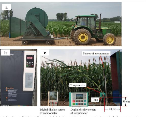
**Fig. 1** Mobile wind machine used in this study. The system included **a** the supporting structure and electric turbofan, **b** a frequency converter, **c** a plant-fixing structure, digital anemometer, and torquemeter
