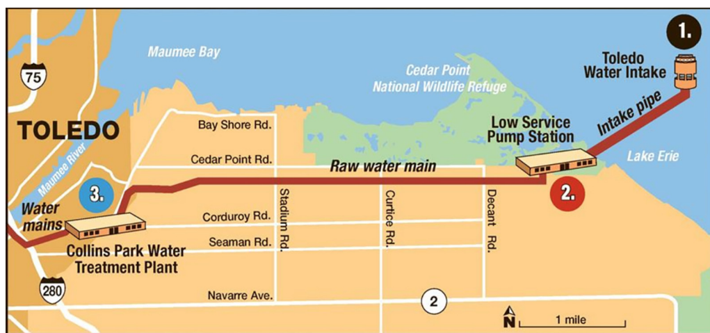
FIG 2 Schematic of the Toledo Collins Park Water Treatment Plant pipeline, indicating where water samples were obtained. Water samples were taken from three locations within the treatment system: the intake crib (site 1, “intake”) which carries the water from Lake Erie directly to the plant for treatment, the surge well within the low service pump station (site 2, “surge”) where the water is treated with potassium permanganate, and the raw water that enters the Collins Park WTP following activated carbon treatment (site 3, “raw”). (Adapted from reference 49 with permission.)
