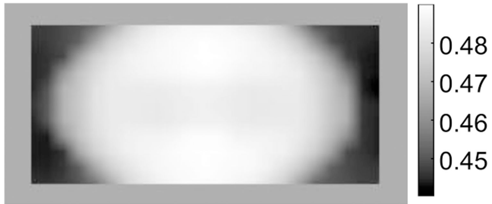
Figure 3: Cross-basis regularization \gamma map for cross-talk reduction.
