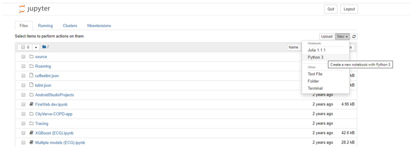
Fig 5. The files and folders tab seen when launching Jupyter notebooks locally. A new notebook is created by selecting the new dropdown option and choosing the required language.
