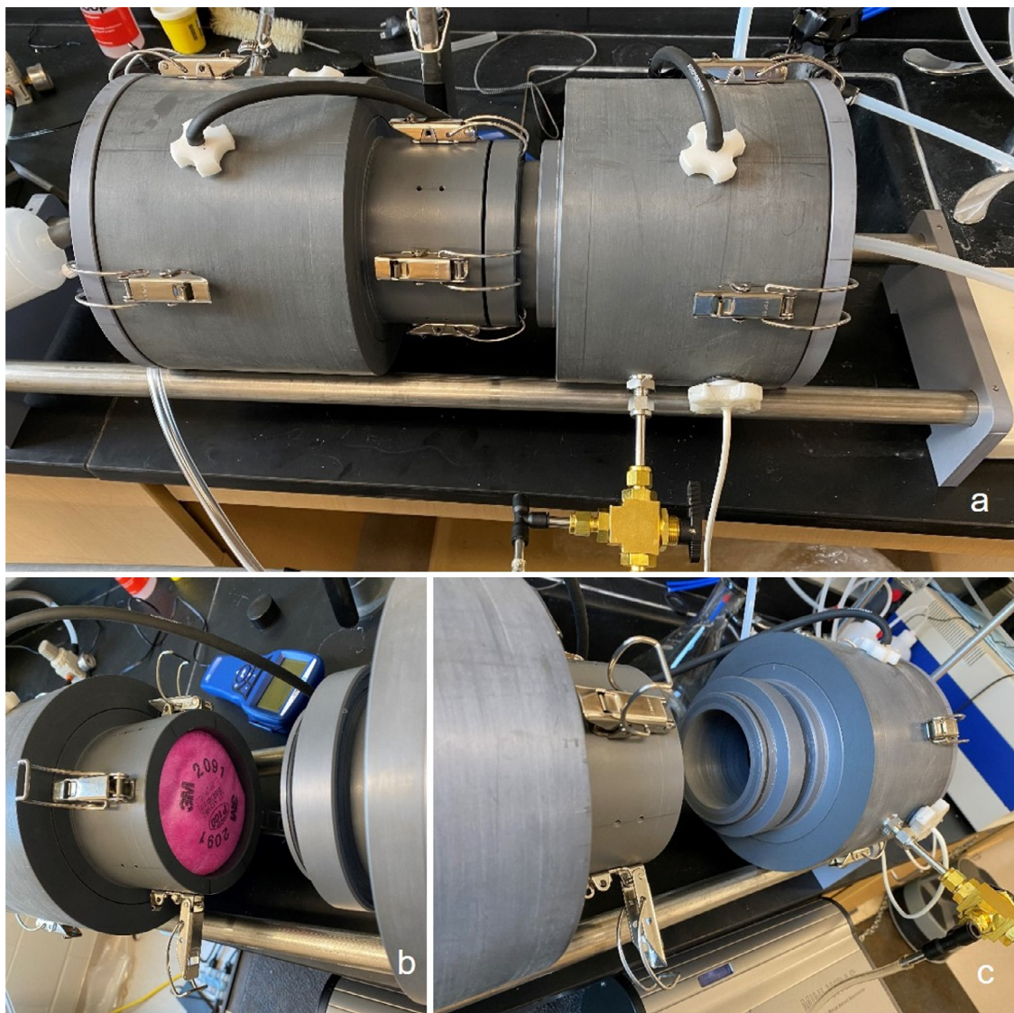
Fig. 2. Customized PVC Exposure Chamber for Challenging the Filter Samples: (A) closed chamber; (B) left side of the chamber holding the test filter; (C) right side of the chamber that secures the filter.
