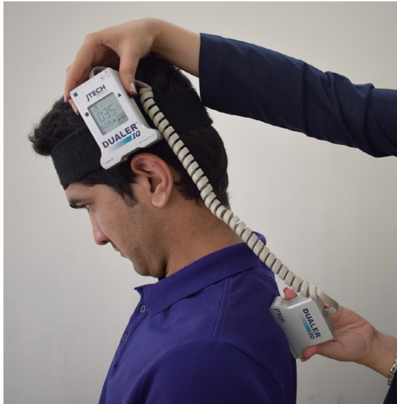
Fig 1. Cervical range of motions measurement in sagittal plane using dual digital inclinometer. Two sensors were used to assess flexion and extension range of motion in 3 trials as the subject was sitting on the chair.
