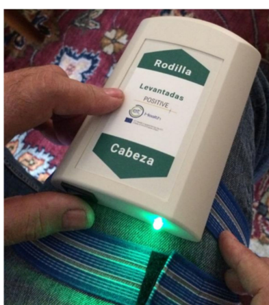
Figure 6. Second version of the sensor casing. The sticker on the sensor reports the correct orientation of the sensor with the help of two tags: “Rodilla”, which is the Spanish word for knee, and “Cabeza”, which is the Spanish word for head.
