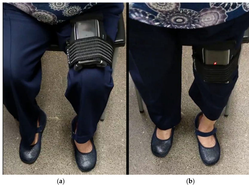
Figure 2. Position and alignment of the sensing device on a subject's thigh. (a) The wearable sensor is placed on the subject's thigh longitudinally aligned with her femur. The sensor is tightly attached to the subject's thigh with a Velcro strap to prevent it from sliding. The LED in the sensor is turned off when the subject is sitting; (b) and it is turned on every time a valid SiSt transition is detected.
