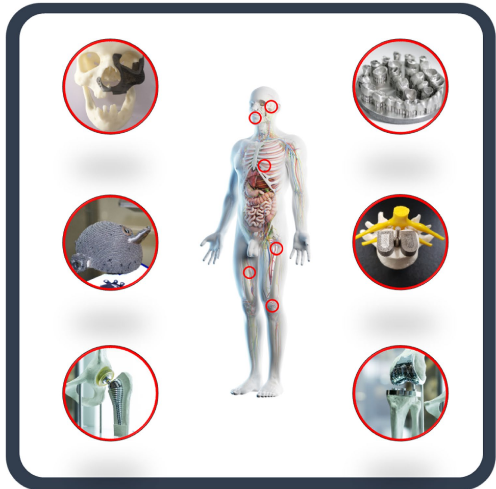
Fig. 1 Schematic diagram of the biomedical application of additive manufacturing of biometals includes cranial prosthesis, dental implants, acetabular cup, interbody fusion cage, hip prosthesis and knee prosthesis
