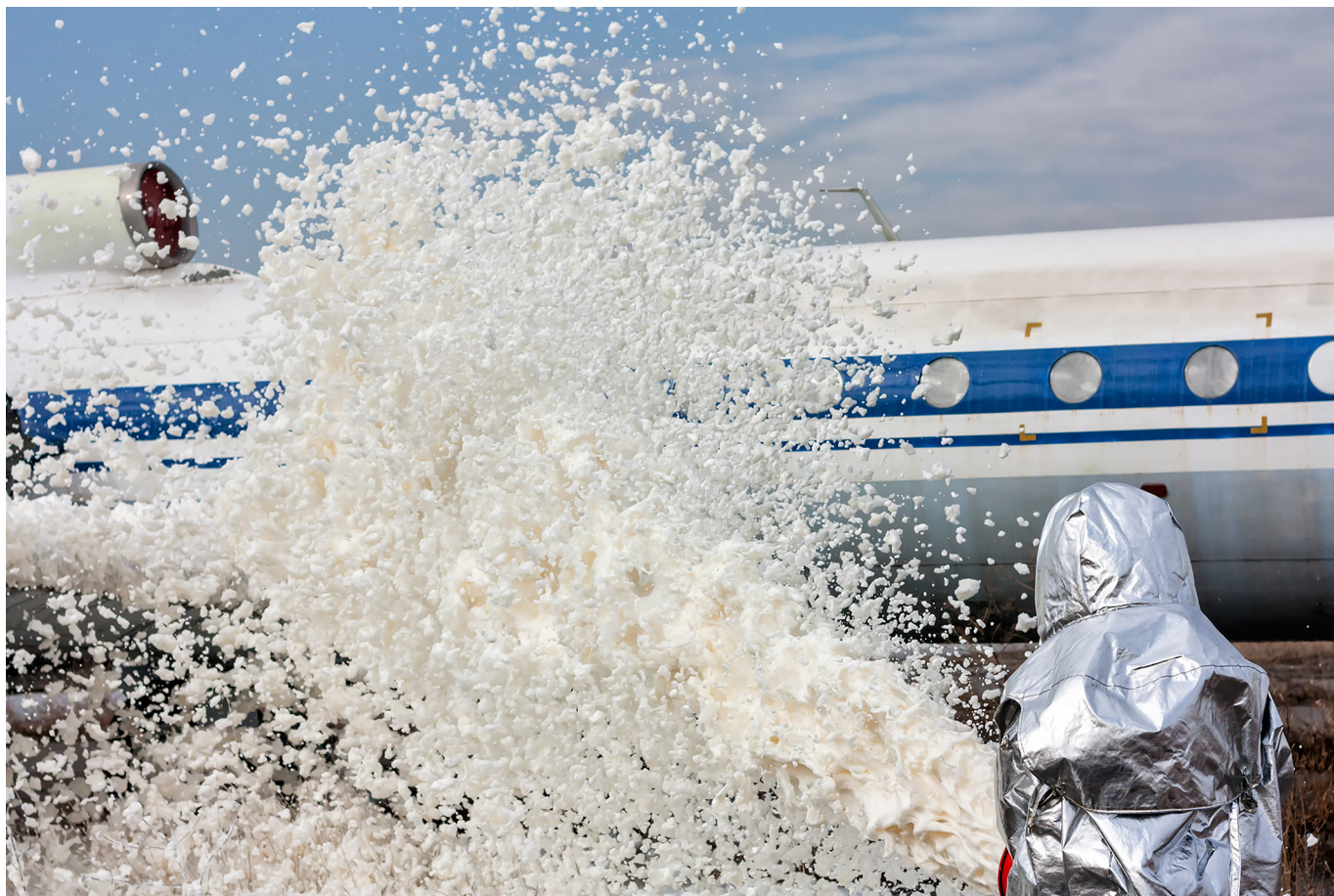
The same chemistry that makes PFAS so persistent in the environment also enables them to quickly extinguish fires. Firefighting foam spreads and forms a film over the fire, smothering the flames and cooling the fuel. Image: © Dushlik/Shutterstock.
