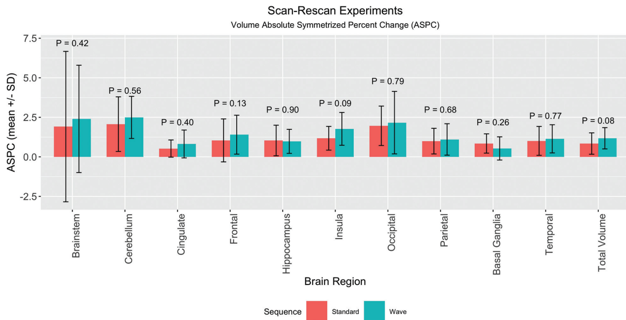
FIG 2. Barplot summarizing the results of the scan-rescan experiments in 10 healthy volunteers. The graph compares the mean and SD of the ASPC of the same sequence (ie, Wave compared with Wave, and standard compared with standard). Each sequence was acquired in different parts of the same scan session (see Materials and Methods for more details). The comparison of the Wave and Standard ASPC was not statistically different for the brain regions studied using a paired t test.
