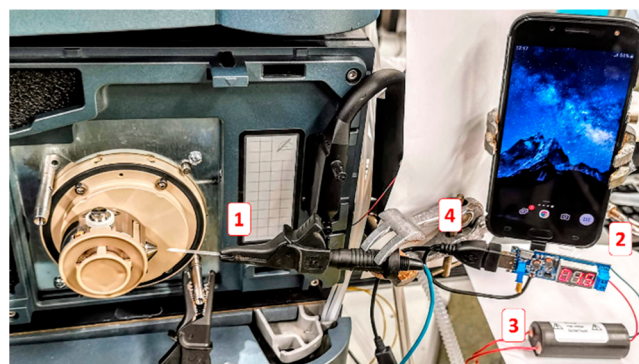
Figure 1. Instrumental setup of an OTG micro-USB phone connected to an adjustable DC/DC USB transformer board coupled to the positive HV generator connected to the coated blade via a toothless crocodile clamp for CBS ionization: (1) crocodile clamp fixing a blade, (2) DC/DC USB transformer board, (3) HV generator module, (4) micro-USB power supply.
