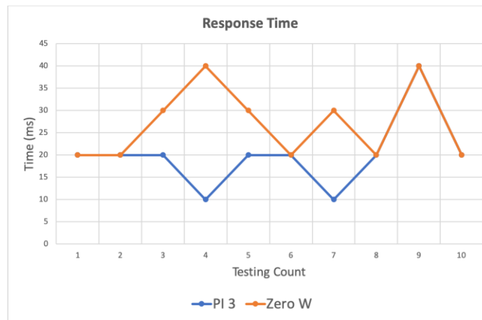
Figure 9. Response time of publish/subscribe for PI 3 and Zero W. The blue line shows that PI 3 is both a publisher and a subscriber. The orange line shows that Zero W is both a publisher and a subscriber.
