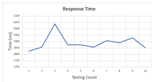
Figure 15. Response time of publish/subscribe between different devices after logical control of gateway. A Zero W as the SDC publishes a message, and then the other Zero W as the TDC subscribes a message.
