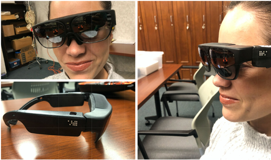
Fig. 5 ODG R7 HMD—non-wired HMD with a semitransparent display, Android-based OS, head gestures, and voice control
