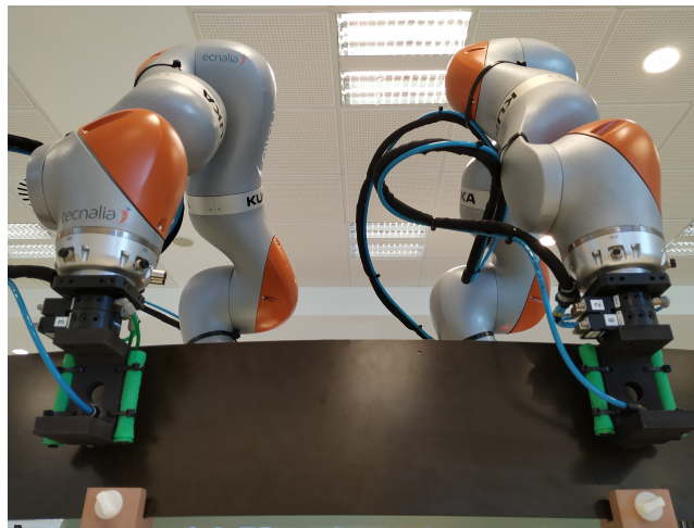
Figure 6. Set-up with two Kuka LBR iiwa robots.
