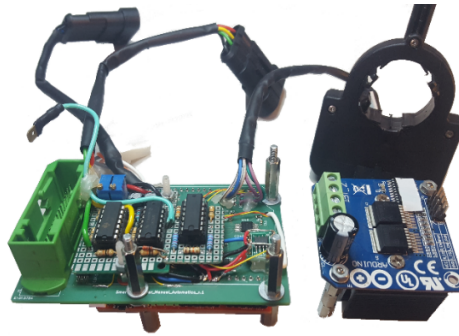
Figure 19. Current state of the Drive-By-Wire hardware.
