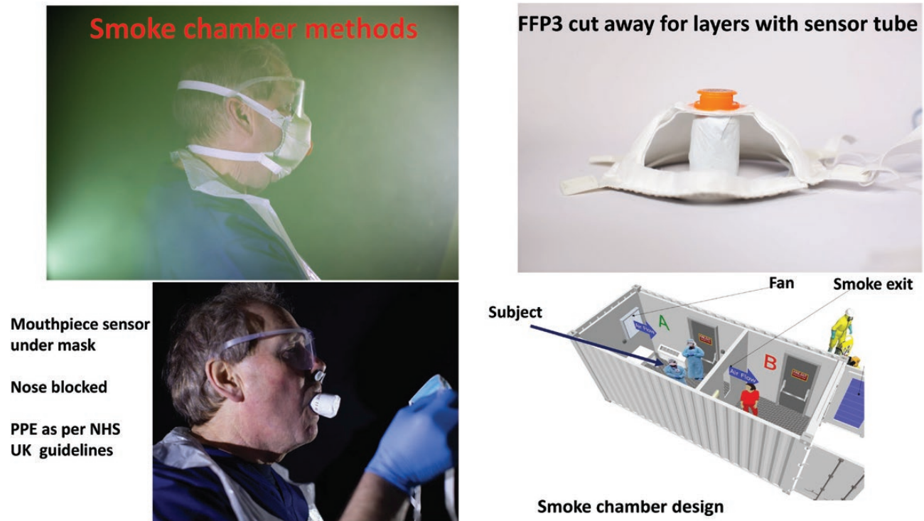
Figure 1. Smoke chamber design.
