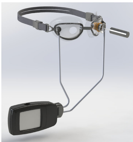
Figure 1. Excursion MPD, an adaptation of the MPD that allows for IOP measurement while negative pressure is active, which includes the goggles and the pressure-modulating pump with crush-resistant tubing that permits independent negative pressure settings for each eye.
