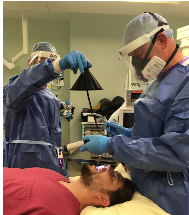
Figure 1 Simulation of aerosol measurement approach within operating theatre environment. The sampling funnel was positioned 0.5 m above the source of aerosol in the airway management zone allowing a sampling stream of air ( 1 \text{ l.min}^{-1} ) to be routed to the optical particle sizer.
