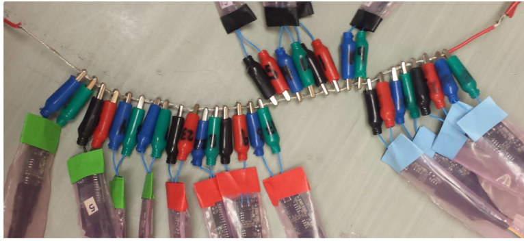
Fig. 5. Test set-up where all of the ACE1 cables were connected to the same voltage source and 100 frames of data were collected. Inputs to the ACE1 current source were grounded.
