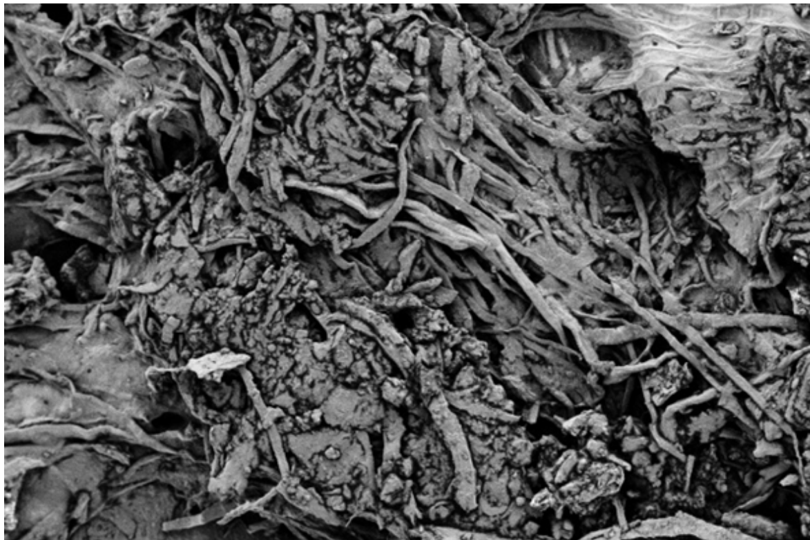
Figure 8 SEM micrograph of FSS char
