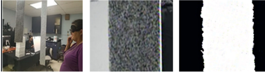
Figure 6. Example of a subject performing the test ( left ), the unfiltered view of a suspended target ( center ), and the distance-filtered view ( right ). The center and right images are from the video output device monitoring the settings.
