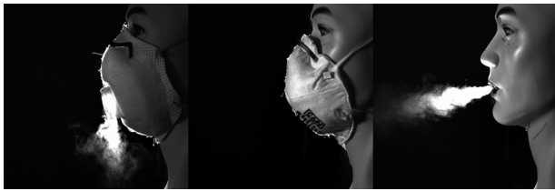
FIG. 2. Still images extracted from the video footage of the mannequin exhaling with an exhalation valve (left), no exhalation valve (center), and no mask (right). The original video footage was captured at 125 FPS. Multimedia view: https://doi.org/10.1063/5.0031996.2
