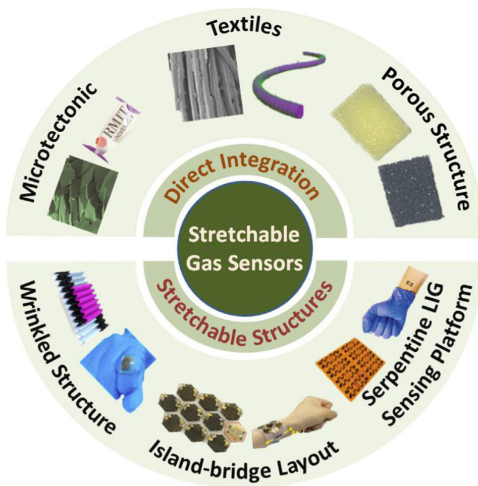
Fig. 1. Stretchable gas sensors enabled by direct integration of gas-sensitive nanomaterials onto the stretchable substrate (template) or by the exploration of stretchable structures. The stretchable substrate template in the former can be thin films (with a microtectonic sensing layer), textiles, porous (fibrous) structures. Reprinted with permissions from Refs. [68-70]. The commonly used stretchable structures in the latter include wrinkled surfaces, island-bridge layouts, strain isolation layers, or their combinations as in the stretchable laser-induced graphene (LIG) gas sensing platform. Reprinted with permissions from Refs. [71-73].
