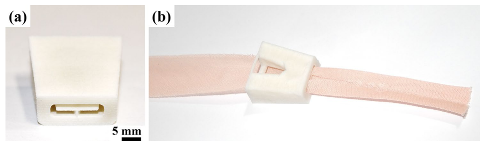
Fig. 8 a Bias tape maker made by SLS/PA12 used for b folding cloth. Model designed by ongaroo user from Thingiverse repository [118]
