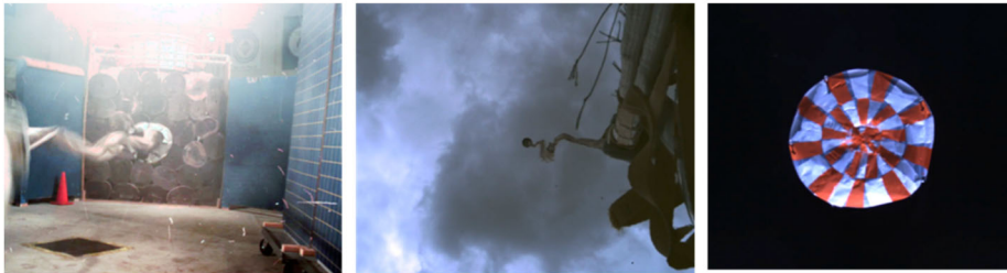
Fig. 39 EDLCAM testing. Indoor mortar firing test (left), outdoor mortar firing test (center), and simulated parachute image testing (right)
