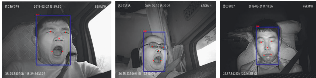
FIGURE 3: Face detection and feature point location using the MTCNN.
