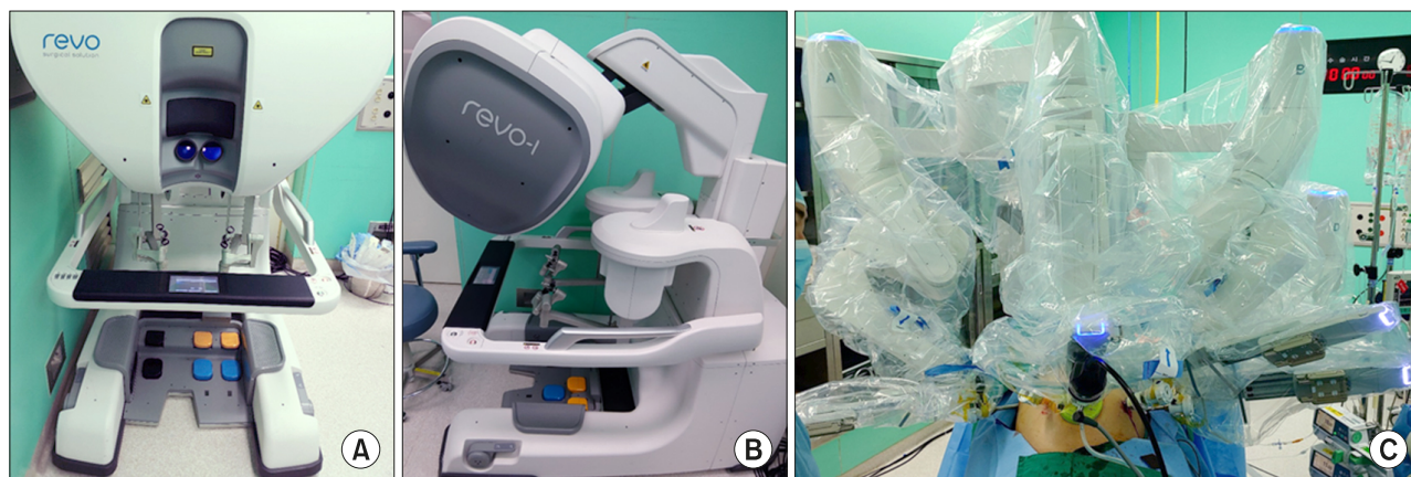
Fig. 1. External view of Revo-i robotic surgical system. (A) Front view of surgical console of Revo-i surgical system. (B) Lateral view of surgical console of Revo-i surgical system. (C) External view after completion of robotic docking to the patient's side ports.
