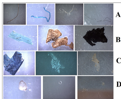
Fig. 8. Example of MP types extracted from sediments ((A) fibers, (B) – fragments, (C) films, (D) beads).
