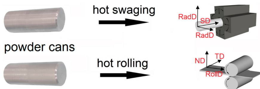
Figure 2. Rolling and swaging geometries used for consolidation of new-generation oxide dispersion-strengthened (ODS) alloys.
