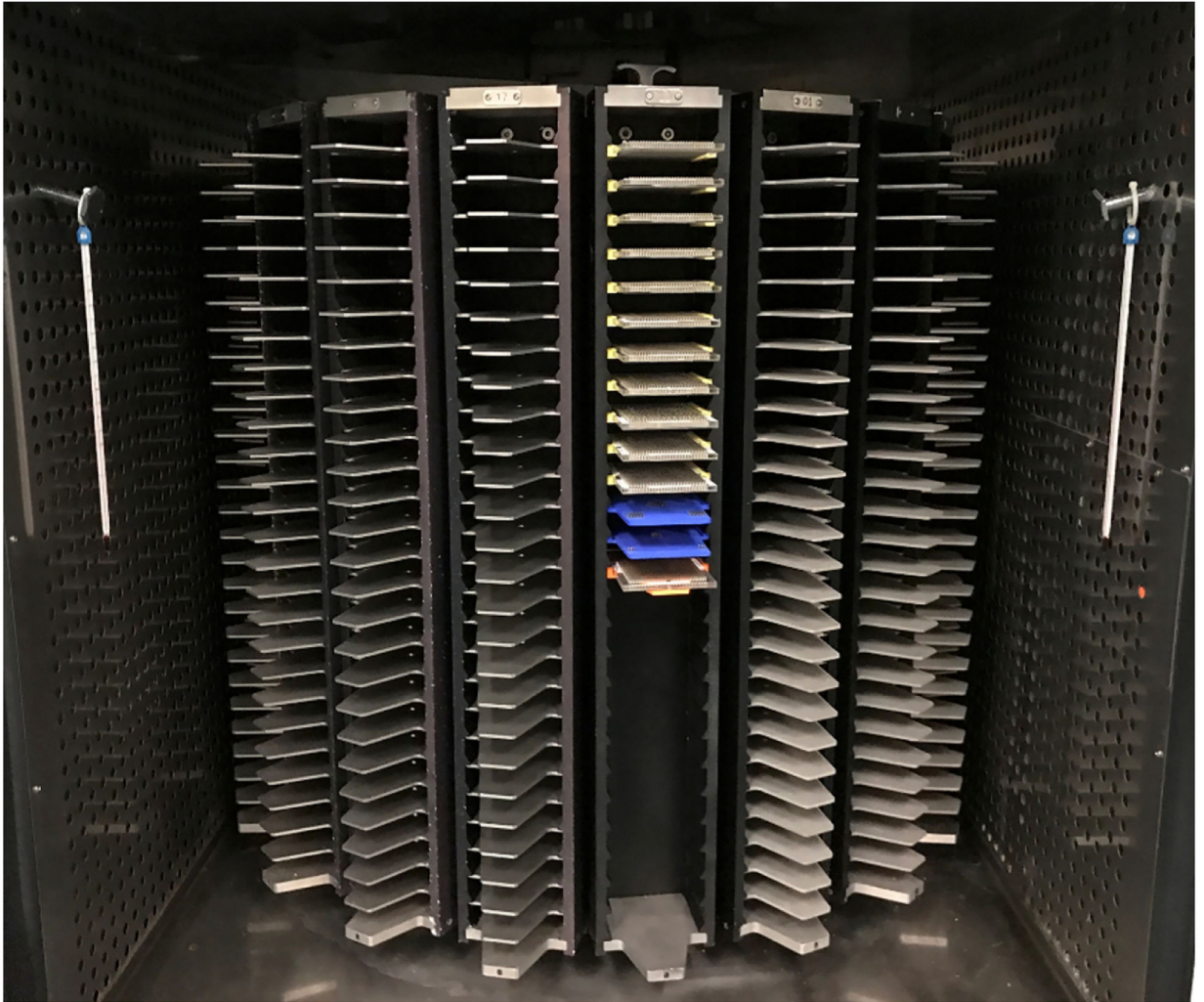
Figure 4. GNF shelf stack installed into GNF robotic carousel.
