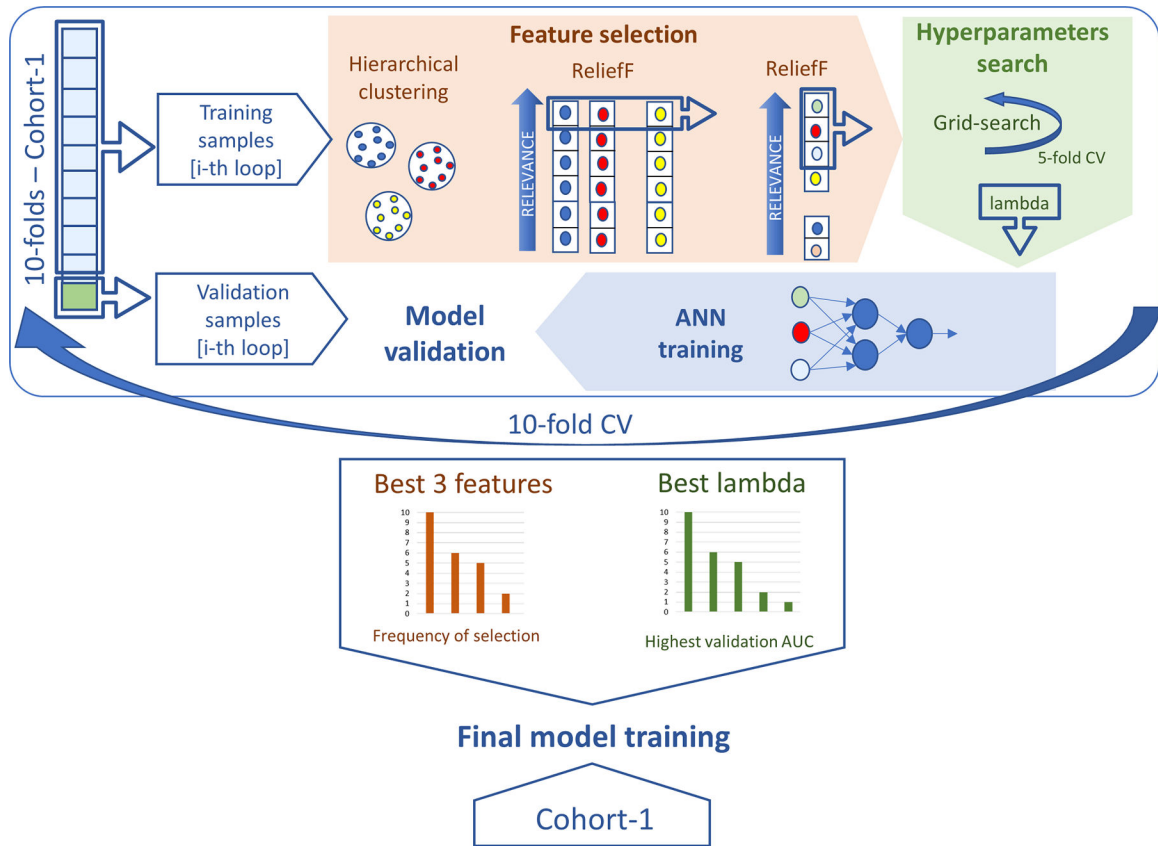
Fig 2. ANN model training. Schematic representation of the methodology adopted in the 10-fold CV to determine the most stable features and the best hyperparameters used to train the final ANN on the complete set of Cohort-1 samples.
