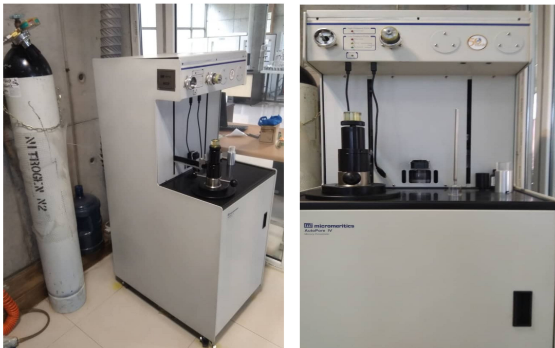
Figure 7. Setup used for mercury injection capillary pressure (MICP) tests.
