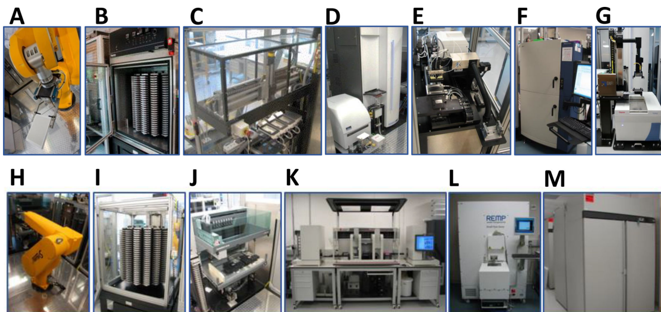
Figure 2. Lead Identification high throughput screening and compound management automation (A) HTS Staubli arm, (B) GNF robotic incubator, (C) GNF pin tool transfer station, (D) Perkin Elmer EnVision and Viewlux plate readers, (E) GNF bottlevalve dispenser, (F) Molecular Devices FLIPR Tetra plate reader, (G) Thermo CellInsight high content reader, (H) Cherrypicker Staubli robotic arm, (I) GNF robotic compound plate carousel, (J) Tecan Freedom Evo span-8 cherrypicker, (K) Beckman Biomek FX, (L) REMP Small Sized Store, (M) Compound freezer farm.
