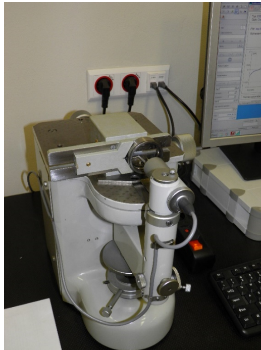
Figure 4. STPP instrument for measuring rolling bearing raceway geometries.
