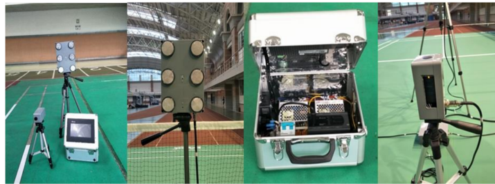
Figure 2. The badminton visual reaction system for badminton training and components.
