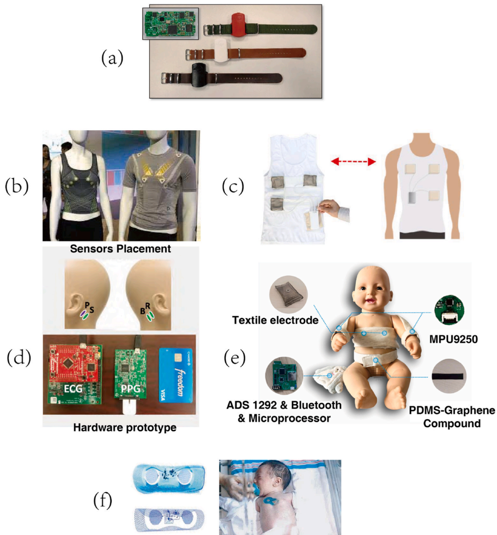
Fig. 2. Prototypes for wearable ECG monitoring: (a) wrist-worn ECG monitor [20]; (b) wearable ECG smart vest system [15]; (c) wearable singlet type with TEs [16]; (d) ear-ECG device [18]; (e) and (f) wearable ECG vest for neonatal monitoring [28,29].
