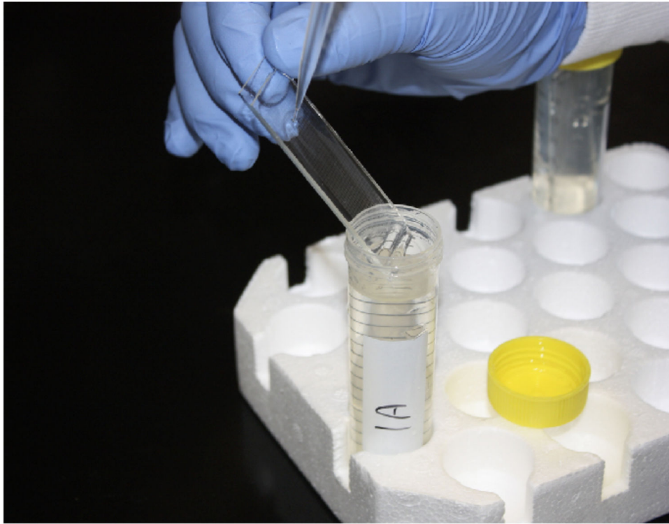
Fig 9. Carefully position the array over a conical of wash buffer and pipette on the array to dislodge beads.
