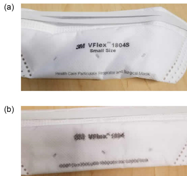
Fig 3. Impact of autoclaving on ink print on 3M 1804 filtering facepiece respirator. A single cycle of autoclaving consistently resulted in varying levels of ink bleeding on 3M 1804 and 9210 masks (a before; b after). Minimal further bleeding of ink was inconsistently observed after additional autoclave cycles. a) Before autoclave. b) After single cycle of autoclave.
