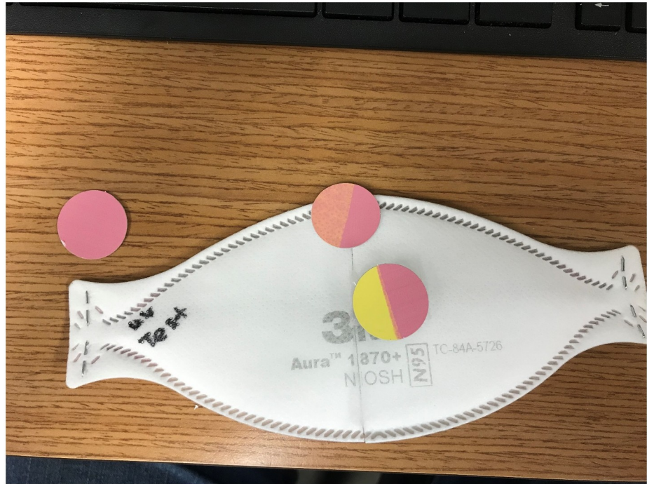
Fig 2. Penetration of UV-C through N95 masks. The degree of UV-C penetration through a layered N95 mask was demonstrated using photochromic UV-C Dosimeter Disks. A 3M 1870+ Aura respirator mask was cut in half, and dosimeter disks were placed directly on top (left disk), half-way under the first fabric layer (top center disk), or half-way under the thick middle layer (lower central disk) of material. A color change from yellow (unexposed) to deep pink was achieved on exposed portions of all disks. The lighter orange color, consistent with reduced UV-C exposure, was revealed on the disk partially covered by the top layer of mask material during UV-C treatment, while the disk placed half beneath the thick middle fabric layer showed no color change from yellow, indicating a lack of exposure to significant UV-C radiation.
