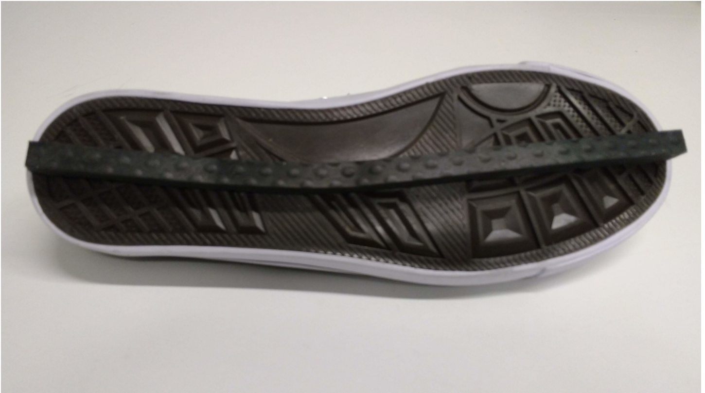
Fig 2. LesSchuh. Shoe with an ankle moment constraint (width of the ridge is 1 cm).
