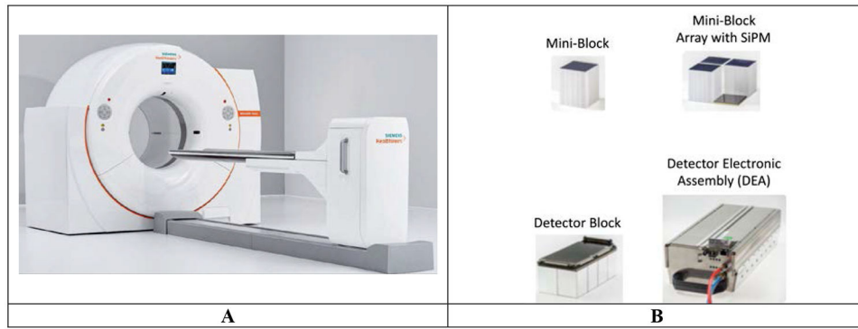
Figure 3: (A) Picture of the Siemens Biograph Vision PET/CT. (B) Picture of a mini-block (5 x 5 array of 3.2 \times 3.2 \times 20 \text{ mm}^3 LSO pixels), a 2 x 2 array of mini-blocks coupled to a 2 x 2 array of SiPMs (each a 4 x 4 array of SiPM channels), a detector block composed of a 4 x 2 array of mini-blocks, and a detector electronic assembly (DEA) of comprising of 2 x 4 array of detectors and associated electronics. Pictures courtesy of Siemens Healthineers.
