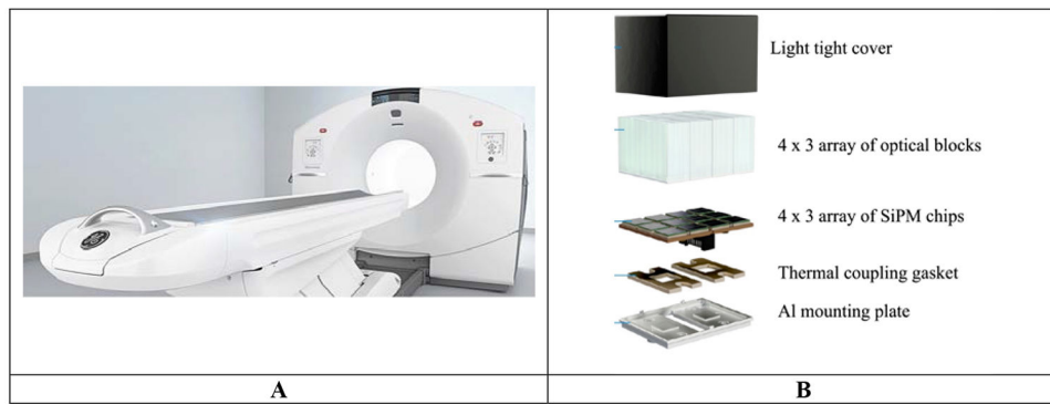
Figure 1: (A) Picture of the GE Discovery MI PET/CT. (B) Picture of a 4x3 array of optical blocks coupled to a 4 x 3 array of SiPM chips [52]. Each optical block is a 4 x 3 array of 3.95 \times 5.3 \times 25 \text{ mm}^3 Lu-based pixels and each SiPM chip is 3 x 2 pixel array with pixel size of 4 \times 6 \text{ mm}^2 .
