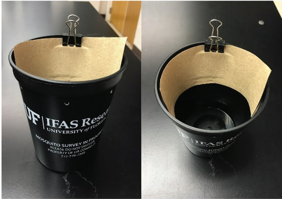
Fig. 1. Basic ovicup made from a black plastic cup, binder clip, and germination paper.
