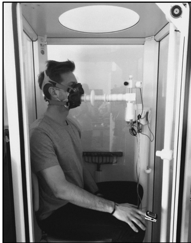
Figure 2. Body plethysmography measurements with spirometry masks.
