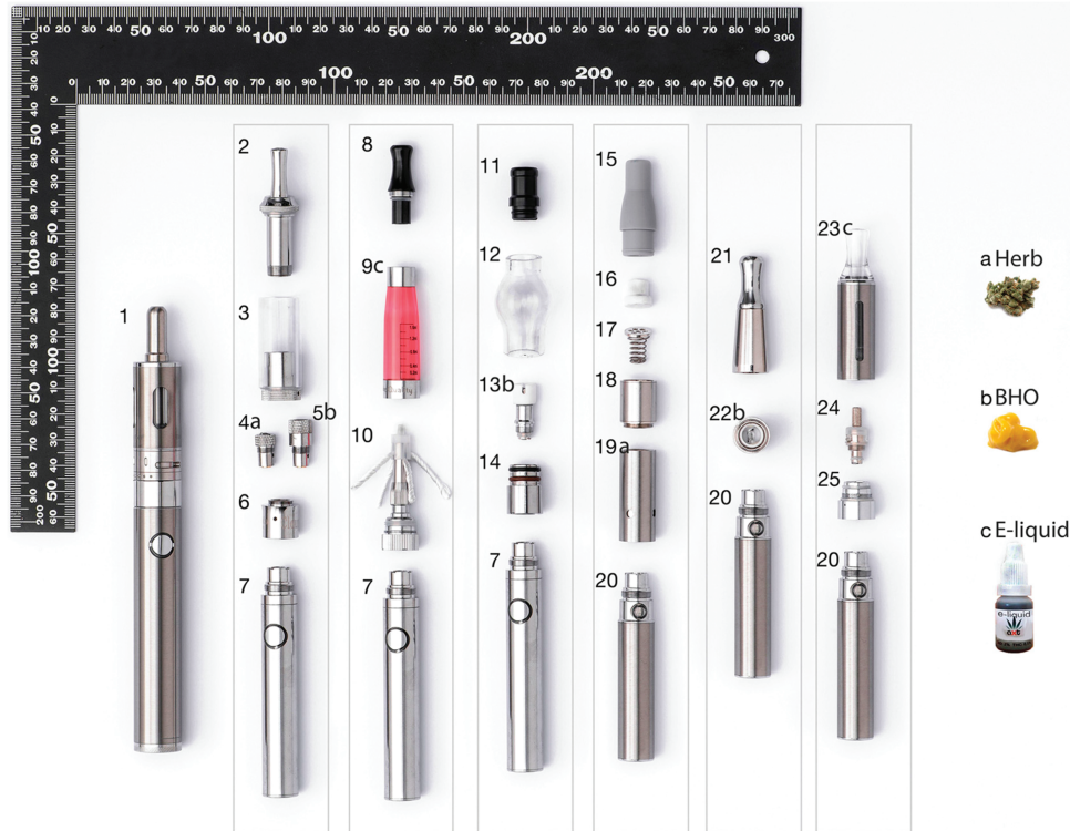
Figure 1. Examples of cannabis vaping devices and their different parts. Some models of vaping devices for use with (a) ground marijuana head tops; (b) cannabis wax (butane honey oil [BHO] concentrate), or (c) cannabis e-liquid. The letters a, b, or c after the numbers indicate the parts of the vaping devices used for herb, BHO, or e-liquid vaping, respectively. 1. Mega electronic cigarette (e-cig) with dual-coil clearomizer, adjustable airflow control ring, changeable resistance coils and high capacity, variable voltage battery. 2–7. Dry herb and wax vaporizer: 2. Spring-loaded mouthpiece; 3. Vaporizer chamber; 4. Dry herb coil head; 5. Wax coil head; 6. Detachable base with air holes; 7. Medium capacity battery. 8–10. See-through clearomizer for e-liquids: 8. Clearomizer tip; 9. Clearomizer tube; 10. Clearomizer coil and four-wick head with base assembly. 11–14. Glass-globe atomizer wax tank: 11. Drip tip; 12. Glass globe; 13. Ceramic heating chamber and coil; 14. Metal core. 15–19. Dry herb atomizer: 15. Soft drip tip (mouthpiece); 16. Ceramic screen; 17. Metal screen and spring; 18. Screens connector; 19. Ceramic chamber and battery connector. 20. Medium size battery. 21–22. Wax coil head atomizer: 21. Metal mouthpiece and wax coil chamber connector; 22. Wax coil ceramic chamber and battery connector. 23–25. Clearomizer for e-liquids: 23. Shell (mouthpiece attached to metal tank with viewing window); 24. Bottom head changeable coil assembly; 25. Battery base connector. a. Marijuana head tops, b. Cannabis BHO concentrate, c. Cannabis e-liquid (mixture of cannabinoid concentrates (cannabis wax), propylene glycol and glycerol). Source: see ref. (40).
