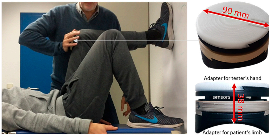
Figure 1. Setting of the manual muscle test (MMT) of the hip flexors with fixed leg including the handheld device. The assistant's leg is fixed against the wall to ensure a stable position also after repeated trials. The tester's forearm is in a rectangular position to the rectus femoris muscle. The handheld device is located between the tester's hand and the assistant's distal thigh to measure the force profile produced by the tester. On the right side, the handheld device with two adapters is illustrated: one for the palm of the tester (white) and one for the limb of the patient (black), which is shaped according to the contours of the limb. Between the adapters, the sensor technology is placed. Dimensions of the handheld device are given in mm.
